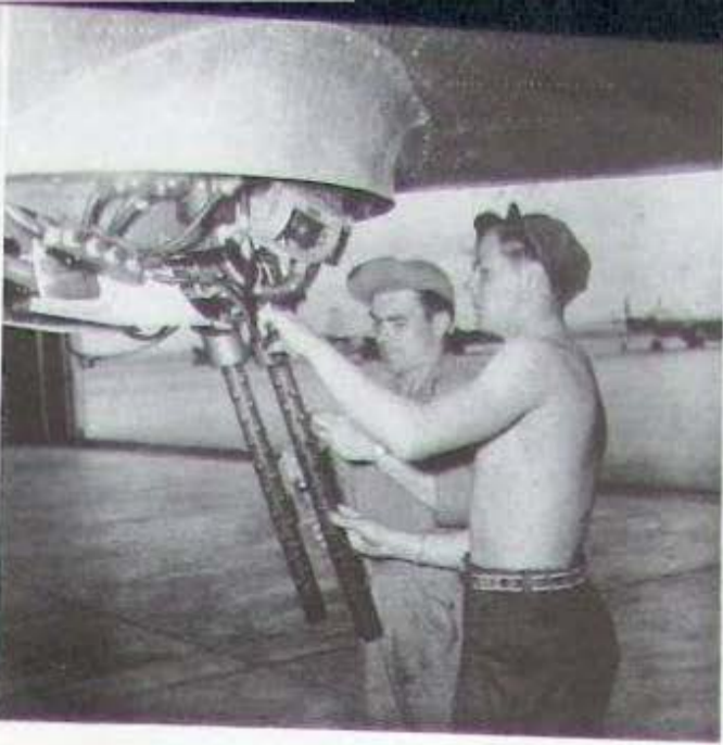
500 hour inspection on lower AFT, 9th BS
