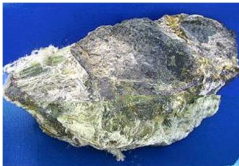
Figure 20.5: Asbestos in the form of chrysotile. You can see fibers of asbestos in the upper left hand corner of the photo. (7)
