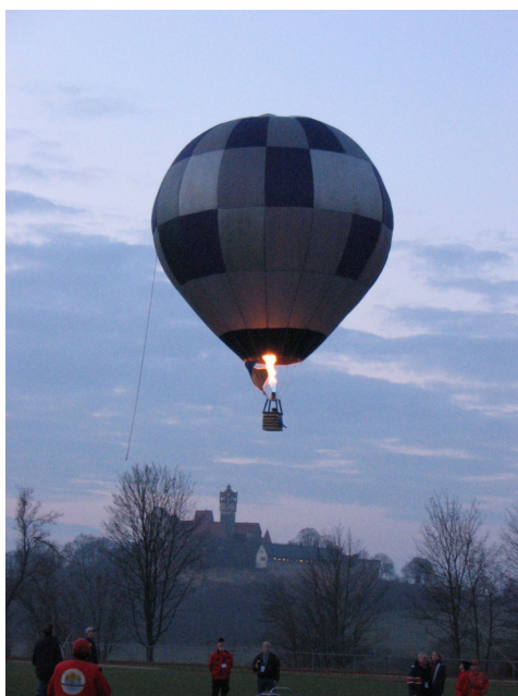
Figure 1.26: A hot air balloon transfers energy in the form of heat from the flame to the air particles in the balloon. The design of the hot air balloon takes this energy and changes it from heat to work. (14)
