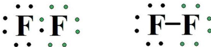
Figure 13.4: We can also show a covalent bond between atoms with an electron dot formula where the shared pair of electrons are the bonding electrons or with the bond represented by a dash. (2)
