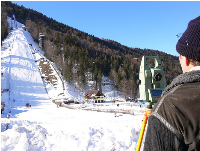
Figure 2.3: Using a laser to make a precise distance measurement. (3)
