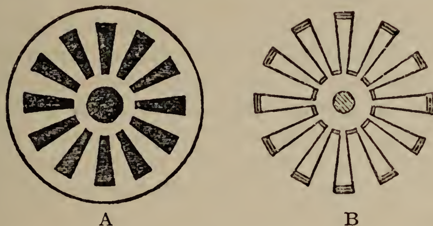
FIG. 15.—THE FIXED (A) AND REVOLVING (B) PARTS OF THE SIREN.
